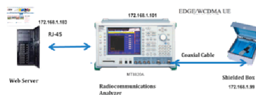
Figure 1. General Test Scenario for EDGE and WCDMA Measurements
